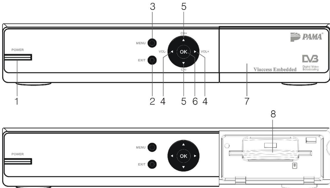
1. **POWER:** Switches between Standby mode and active mode.
